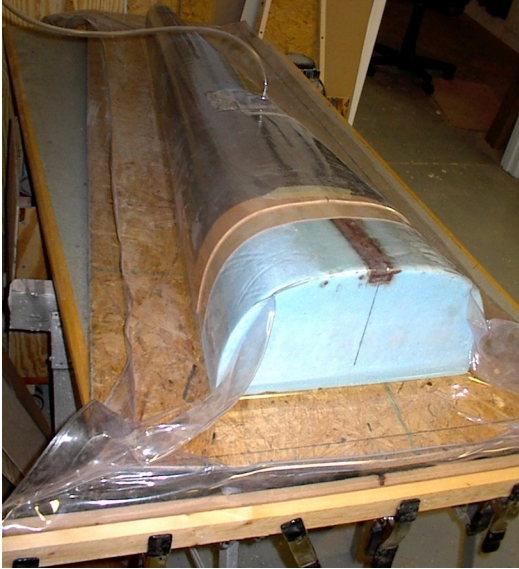
A round back shell over a foam mold, curing in a vacuum press bag
