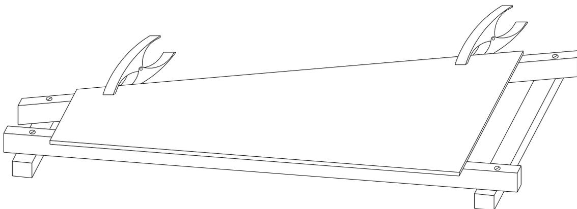
If you will be doing most of the tapering with a hand plane, I suggest gluing the string rib to the first side of the board after you have sanded it smooth. Even with a newly sharpened plane, I have to apply enough pressure that the board needs to be reinforced to keep it from buckling and breaking, especially at the thin end.
