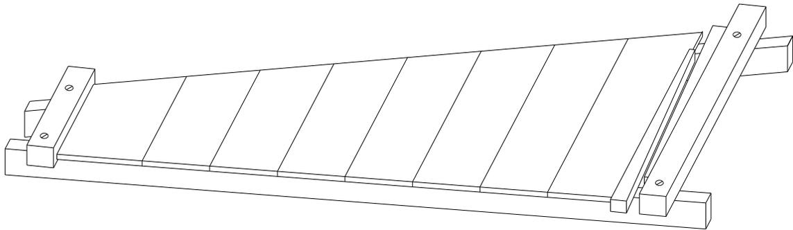
I place the planks on the frame, and move the cross brace at the top up or down so that the two wedges can be slid into place. Check the seams between the planks and make sure they are tight. Fix any gaps with a jointer. At this point I place the sound box on top of the planks to make sure I have allowance all around. I also strike a light pencil line from the treble to the bass end and use it to align the planks during the glue up.
