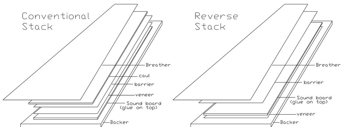
In conventional vacuum veneering, a caul is used on top of the veneer to ensure it comes out flat. In this stack the veneer is usually a bit smaller than the substrate and the caul is a bit smaller than the veneer to prevent it from driving all of the glue out from under the edges of the veneer as the bag is evacuated.
