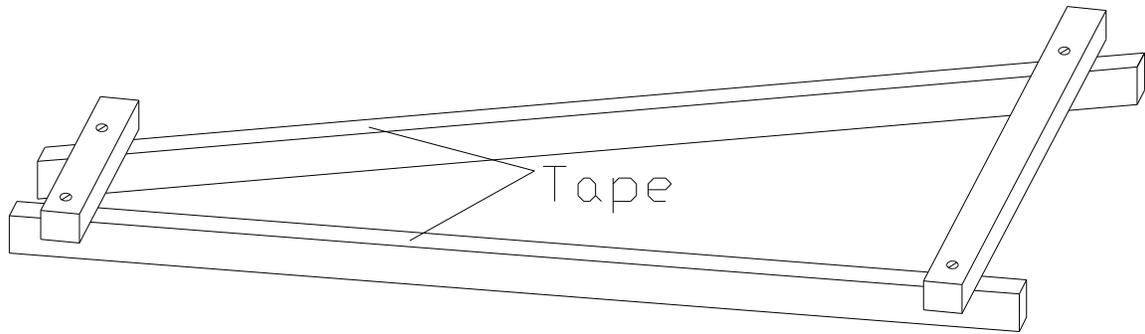
Packing tape on the two long sticks of the frame to will keep the soundboards from being glued on to the frame. I make two long wedges from  $\frac{3}{4}$ " stock - 12" long that taper from  $\frac{1}{4}$ " to  $\frac{3}{4}$ ".
