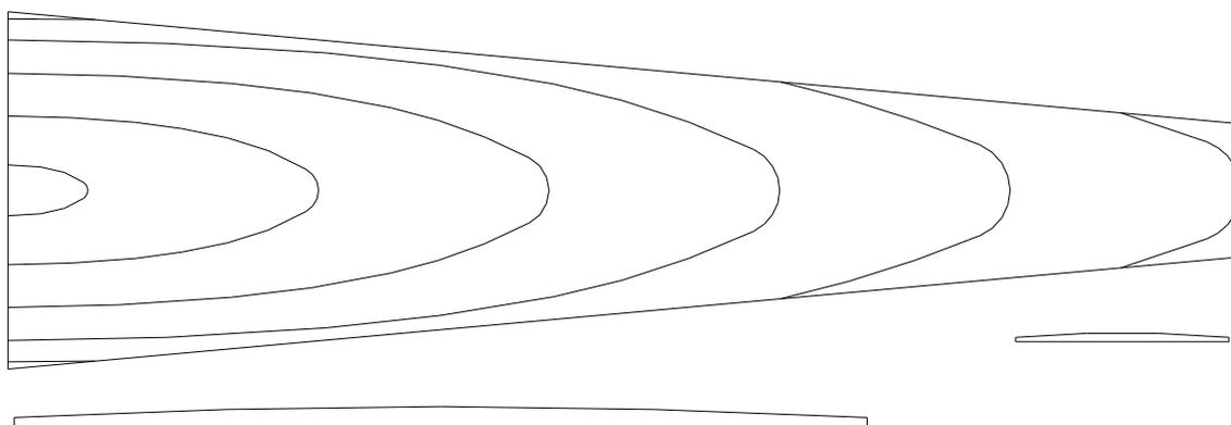
The flat plates below the contour drawing are enlarged cross sections of the board at the bass and treble end. I use a linear taper along the length of the board - midway up the board - the center thickness should be  $15/64''$ . The string ribs have straight line tapers too. The side to side taper on the soundboard is a gentle arc.
