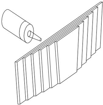
I use yellow carpenter's glue. To spread the glue quickly and efficiently, I "collate" the boards together in an even stack. I use a spring clamp to hold them while I spread the glue on eight or nine edges all at once. After taking off the top and bottom boards (they only need glue on one edge) I flip the stack over, re-clamp and spread glue on the opposite edges.
