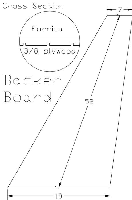
By reversing the conventional stack and placing the veneer between the backer and the substrate, the need for a carefully sized caul is eliminated and the board comes out of the press with a top that is as flat as the Formica it was molded on. I use the flattest, shiniest Formica I can get and cover it with a coat of car wax (that is then thoroughly buffed) to prevent any glue that seeps through the veneer from sticking, gluing the sound board to backer board.
