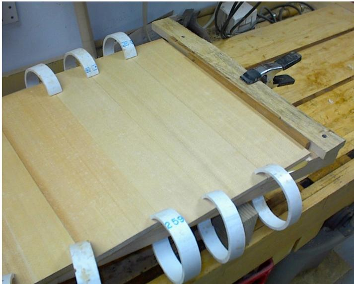
*Photo – The bass end of a soundboard with the planks glued up and wedged in compression. You can see the frame, ring clamps and wedges. The frame is propped above the workbench with 2/4's. The hand spring clamp on the end of the frame board holds a small piece of scrap wood to keep the wedges from falling through the frame*
