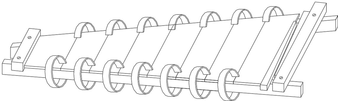
After the glue dries, you should have a soundboard that is dead flat on one side. Take the clamps off and lift the soundboard off of the frame. At this point the soundboard will be alarmingly floppy, so handle it gingerly until the string rib has been glued on.
