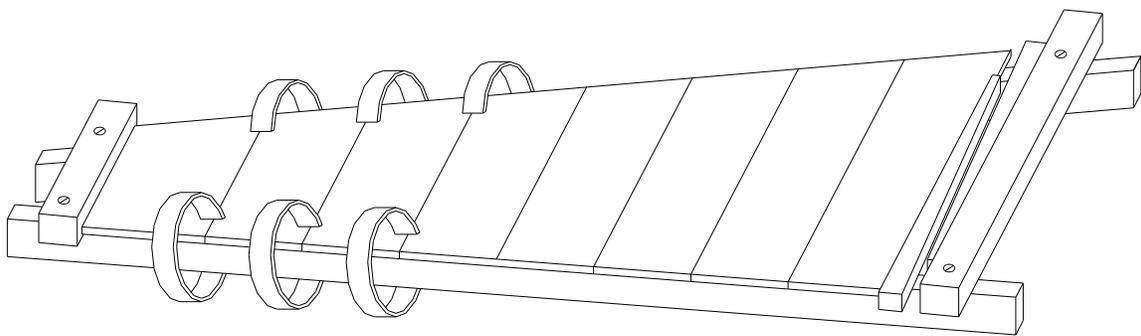
I start placing the ring clamps at the top (treble) end of the sound board. After I have put on the first six clamps or so, I stop and tap the wedges lightly to generate a little more pressure. When I've placed about 2/3 of the ring clamps I'll tap the wedges a second time to increase the pressure between boards. Too much pressure will starve the glue joint. The glue seam at the bottom is 16" long and has a lot more surface area than the joint at the top, so the third function of
