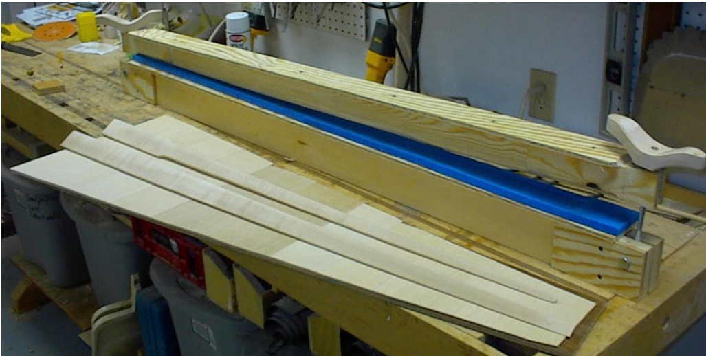
The clamping jig, a soundboard and finished ribs ready for gluing
