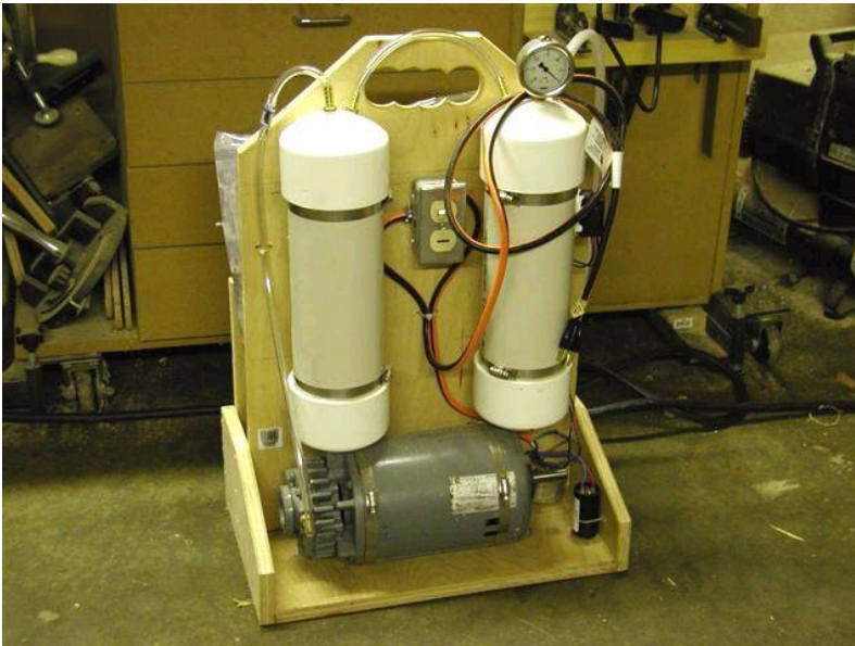
Home built vacuum pump, resevoir and regulator, From www.joewoodworker.com website.
