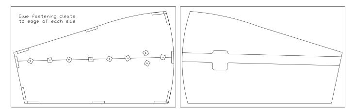
On the opposite side of each side panel (the side that will become the inside of the case) I glue the side rails centered over the cut line. I use screws with plywood pads, through holes predrilled every 4-6 along the "cut line"
