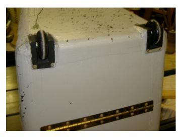
The casters stand about <sup>3</sup>/<sub>4</sub>" proud of the case, and to get it back to level, I mount two rubber bumpers with T-nuts on the bottom panel of the lid so when the case is standing upright it will not have the tendency to fall forward over.
