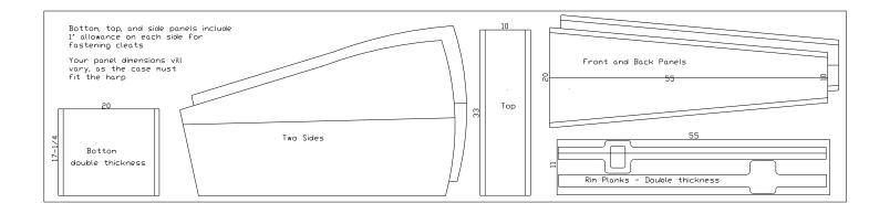
While I am at it, I lay also measure and cut out the bottom and top panels. These panels should also have a one inch allowance on each side to allow me to screw these parts to the sides on the temporary assembly cleats.
