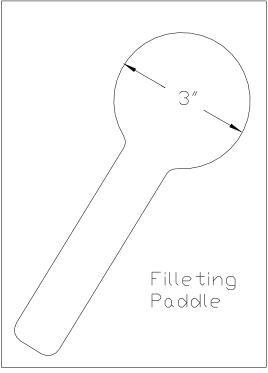
I roll out the 6" wide tape cutting it to length for the 8 corner seams I will be filleting. It is a long reach down into the corner seam near the top, and I find it helps to prop the box 18" off the floor on a few 5 gallon paint buckets. From scrap plywood, I make a several paddles for spreading the epoxy. Make the head so it is about three inches in diameter.
