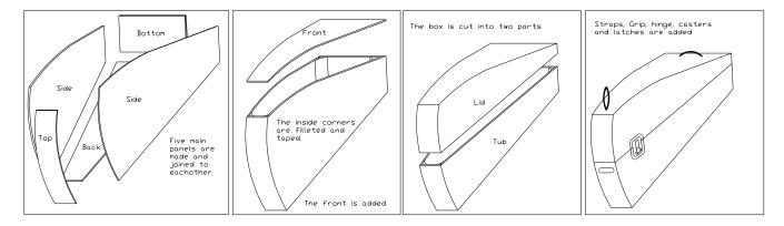
Much of the case strength and durability comes from the epoxy and fiberglass used to join the panels together. These joints are light and very, very tough. To hold the panels securely to each other while making the inside fillets, I use an external cleat that is trimmed off after the inside of the box has been fiberglassed..
